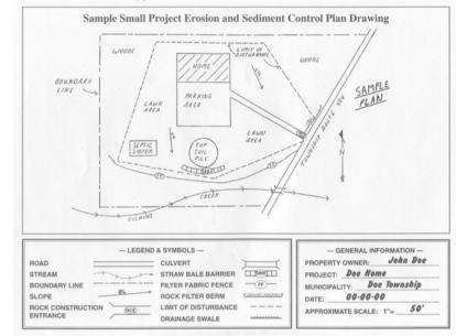
E&S Plans should be site specific and include maps illustrating the project site area, proposed alterations, BMP's for each project phase and a maintenance program for control measures.
